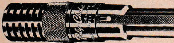
Adjustable shotgun choke. Choke is varied by turning knurled ring.
